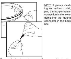
ing an outdoor model, plug the two-pin heater connection in the lower dome into the mating connector in the back box.
